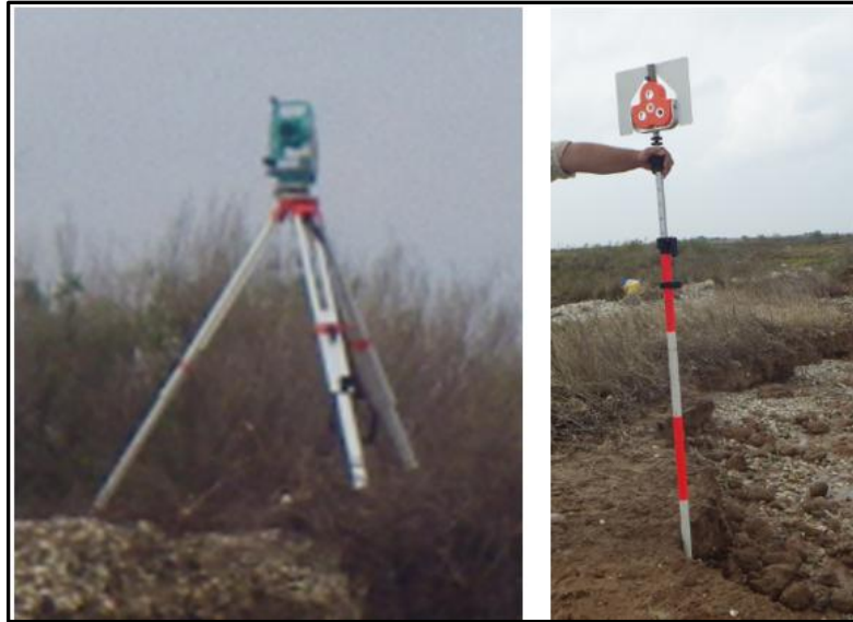
Figure 12. Sokkia 330R Total Station (left) and target prism (right).
