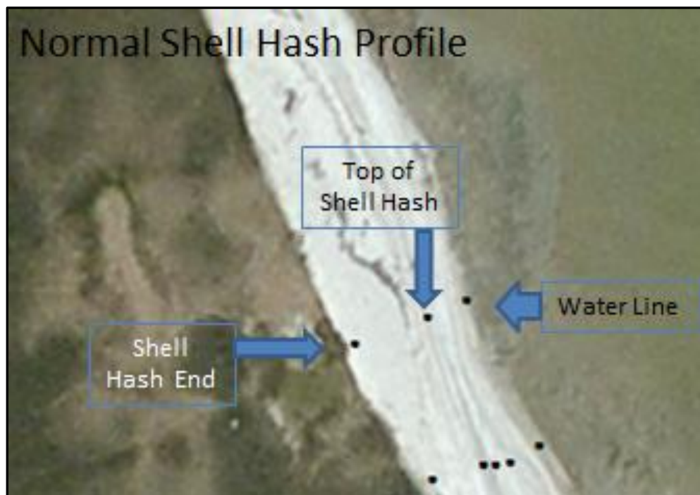
Figure 13. Identified points taken with the total station.
