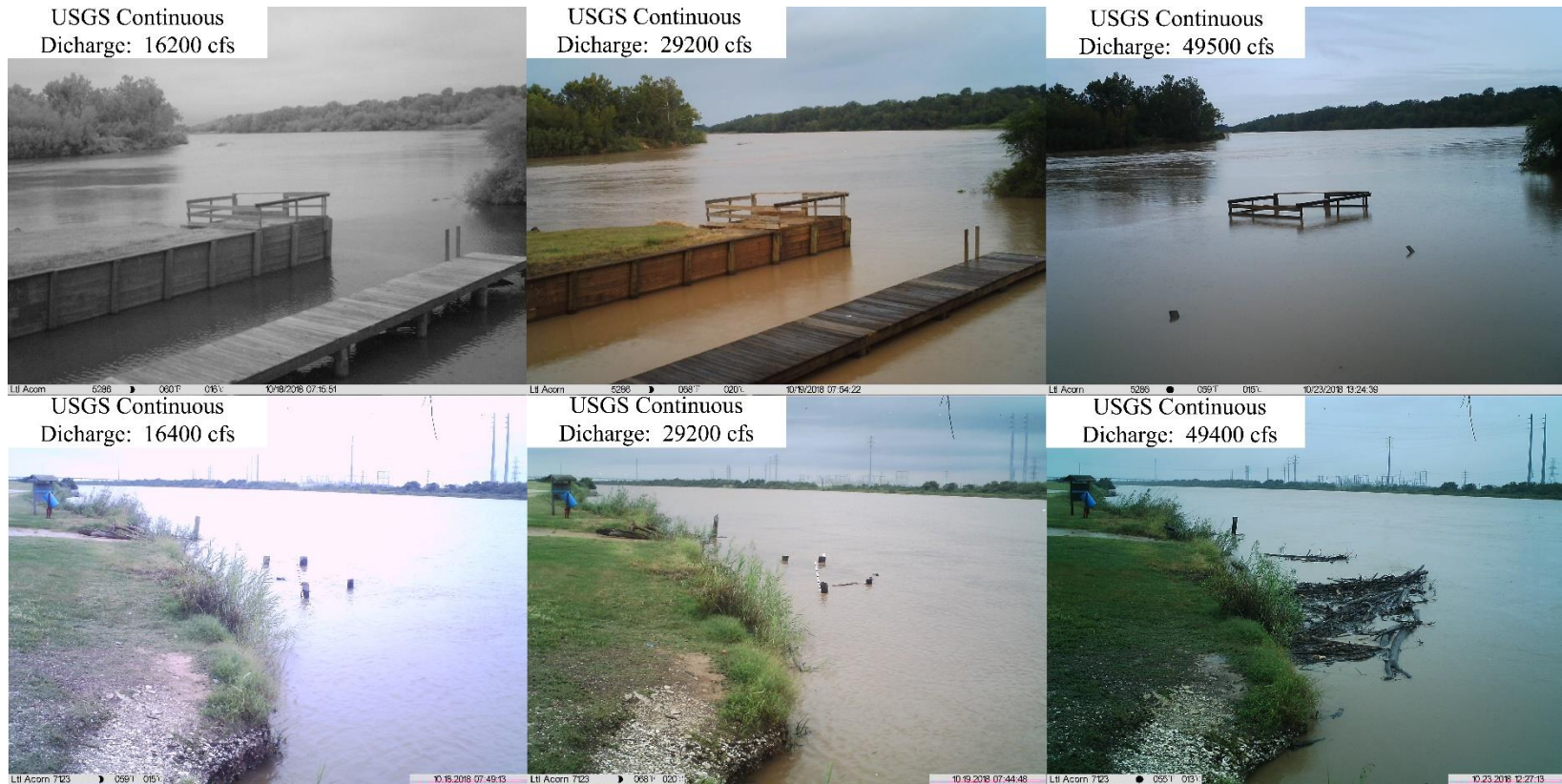
Figure 60. Time lapse photos from Lower (Bottom) and Middle (Top) game cameras between 10/18/18 to 10/23/18. Timestamps at the bottom of the photos are one hour behind actual time. Discharge values in the top left show what was recorded at USGS gage #08116650 at the time the photo was taken.
