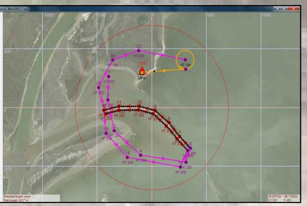
Fig 6. A flying acquisition plan in the Bastrop Bay shows the flying path that includes the launching and navigation part, surveying path along the reef and the navigation part to landin
