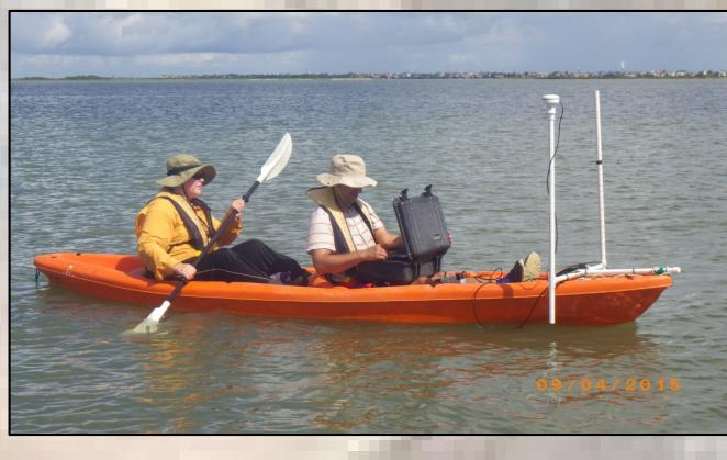
Fig 3. Operating the side-scanning sonar system in shallow water from a kayak.
