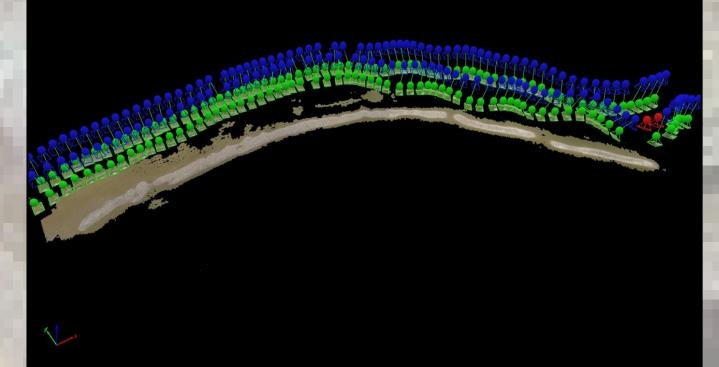
Fig 7. Densified point cloud: green dots indicate where the UAV is, blue dots where the UAV should be at the time of the image capture, and red dots indicate discarded data.
