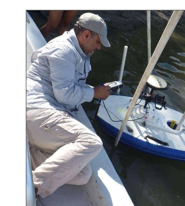
Figure 7. EIH staff measuring water surface elevation using DGPS.
