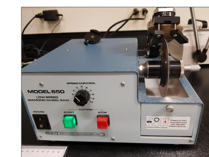
Figure 6. Low-speed diamond wheel saw used for shell sectioning.
