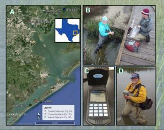
Figure 1. (A) Map of Galveston Bay displaying site locations and marsh type; (B) Collecting water samples at a created saltmarsh; (C) Hach DR/890 Colorimeter; (D) Using YSI handheld monitoring device
