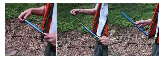
An increment borer is used to determine the age of a tree. The borer is compact so it can fit into a pocket of the vest and is easily assembled.
