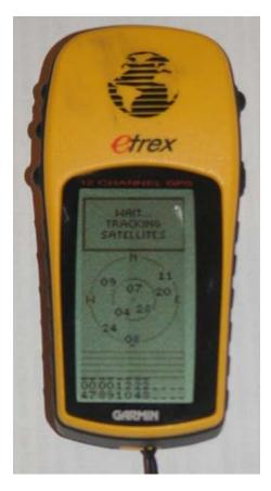
The GPS unit above is a Garmin etrex that provides the user with the necessary tools to obtain latitude, longitude, elevation, and the ability to mark and save routes. GPS is a used for a variety of purposes. Its uses are found everywhere from the military to inside peoples' cars as a navigation system.
