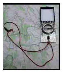
A compass is used to determine direction. Often times it is used to determine which direction the slope of a hill faces. This information is useful when deciding which vegetation will grow best on a particular site. A compass really comes in handy if you get lost in the woods.
