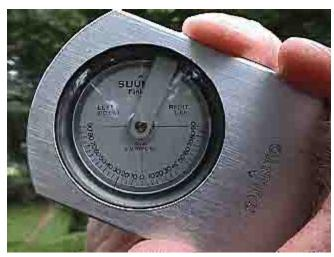
A clinometer is used by foresters to measure the height of a standing tree. It works using principles of angles and geometry.
